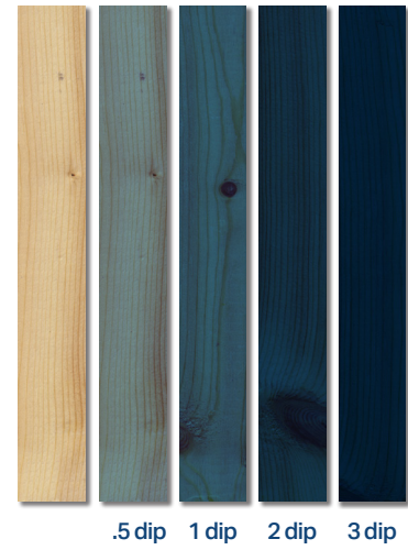
fig. 2: saturation levels of indigo relative to how many times the wood is dipped into the indigo dye; a similar exercise would be displayed inside the pavilion to describe the dyeing process.
